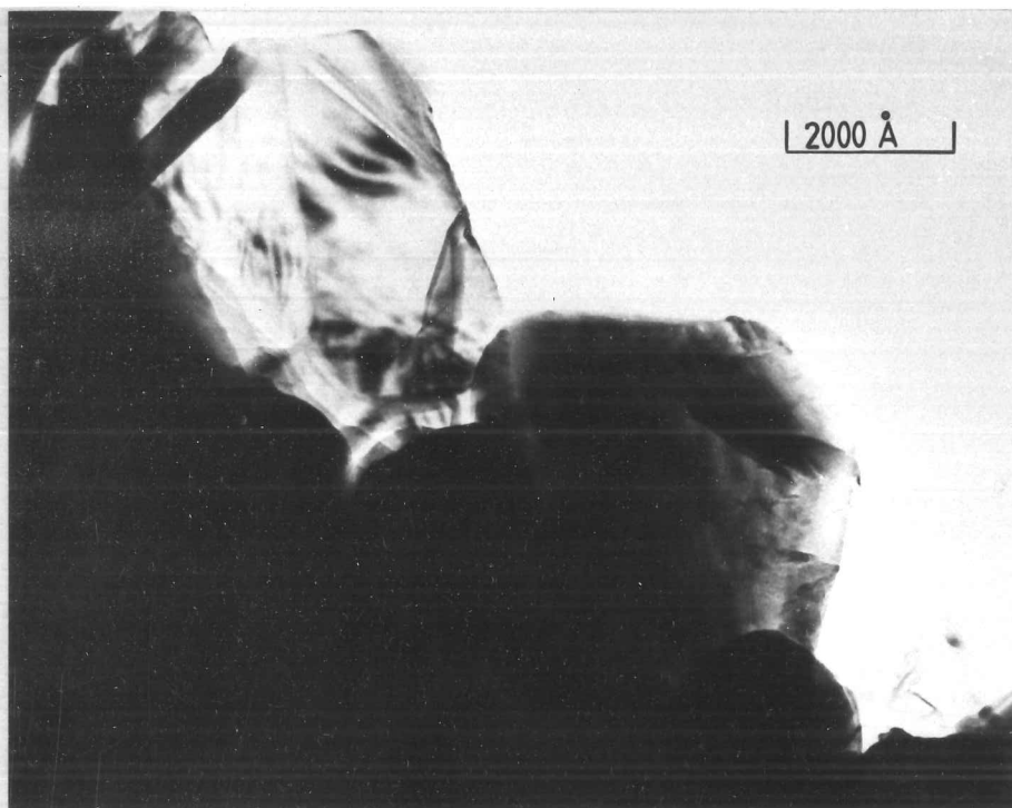
Figure 5.1c : bright-field micrograph of graphitic boron nitride showing large platelets containing large (several hundred Å) uniform-thickness areas.
